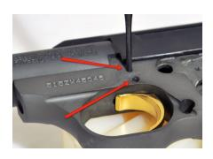
6. Install the Set screw into the trigger, leaving it so that the set screw is on the face side of the trigger. This allows the trigger to be inserted and assists with the installation of the screw.
